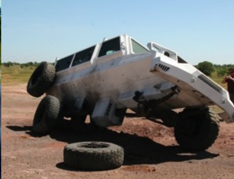
Undamaged SETS APC body structure after 8kg hull shot testing
